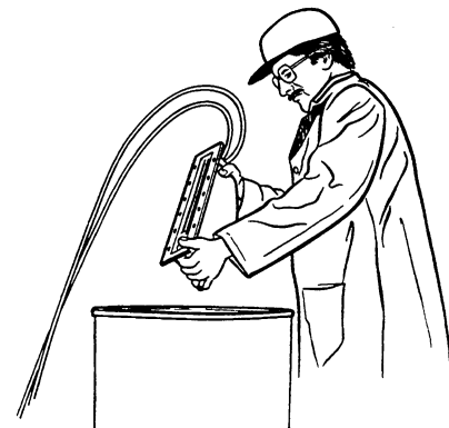
Install a plug in the air vent valve and put a cap on one of the aftercooler water hose tube. Attach regulated air pressure to the other water hose tube. Pressurize the core to 206 kPa (2 bar) (30 PSI) and submerge the aftercooler in water. Inspect for any air leaks. If there leaks or damage, the aftercooler must be replaced.
