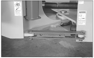
Park machine on a level surface and lower bucket to ground. Put articulation lock in LOCKED position.
