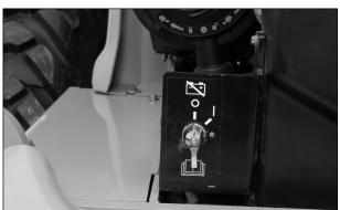
The master disconnect is located under the hood on the left read side of the machine. Raise the hood put master disconnect switch in OFF position. Remove both battery covers and disconnect batteries from the machine.
