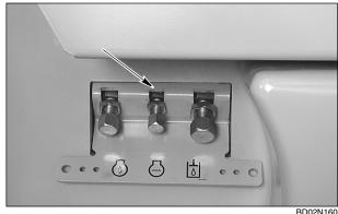
Put a container capable of holding at least 22.7 liter (6.0 gallon) below radiator drain. Remove radiator cap. Remove cap and drain coolant into container. Install cap after coolant has drained. Install radiator сар.
